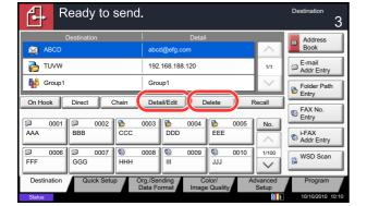
**NOTE:** When selecting [On] for Entry Check for New Destination (*page 9-45*), the confirmation screen appears. Enter the same destination again and press [OK].
